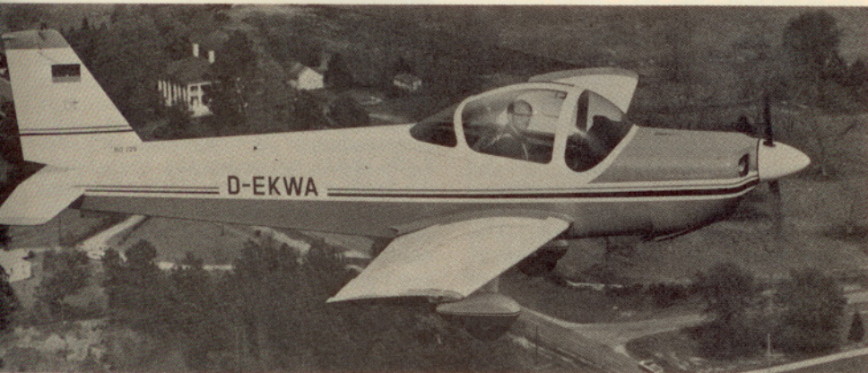
The 160 h.p. Monsun in flight over west Georgia. Dave Forrest is flying from right side so the control stick is in his right hand. The nosewheel is retracted, giving the plane 6½ to 7½ m.p.h. extra speed.
