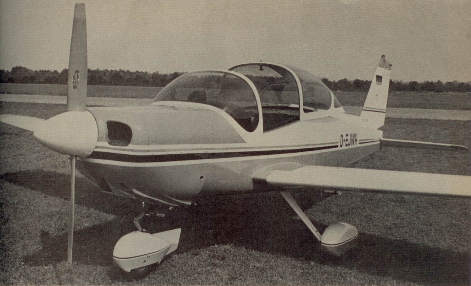
The 150 h.p. Monsun . Note the faired nosewheel on 160 h.p. model retracts.
